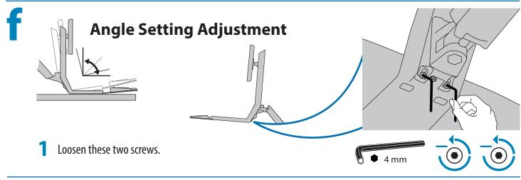
**2** Loosen or tighten this bolt to adjust tilt to desired angle.
