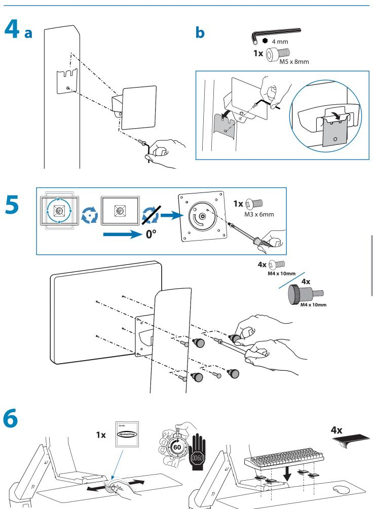
NOTE: Leave enough slack in cable to allow full range of motion.
