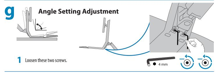
2 Loosen or tighten this bolt to adjust tilt to desired angle.
