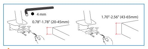
Warning: Because mounting surface materials can vary widely, it is imperative that you make sure mounting surface is strong enough to handle mounted product and equipment.
