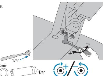
3 After desired tilt is achieved, retighten these two screws to secure.
