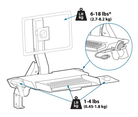
\*The Combo Arm can be modified to mount displays up to 25 lbs (11.3 kg), however display lift and tilt motion will not be possible if this option is chosen. Refer to special instructions on page 7.
